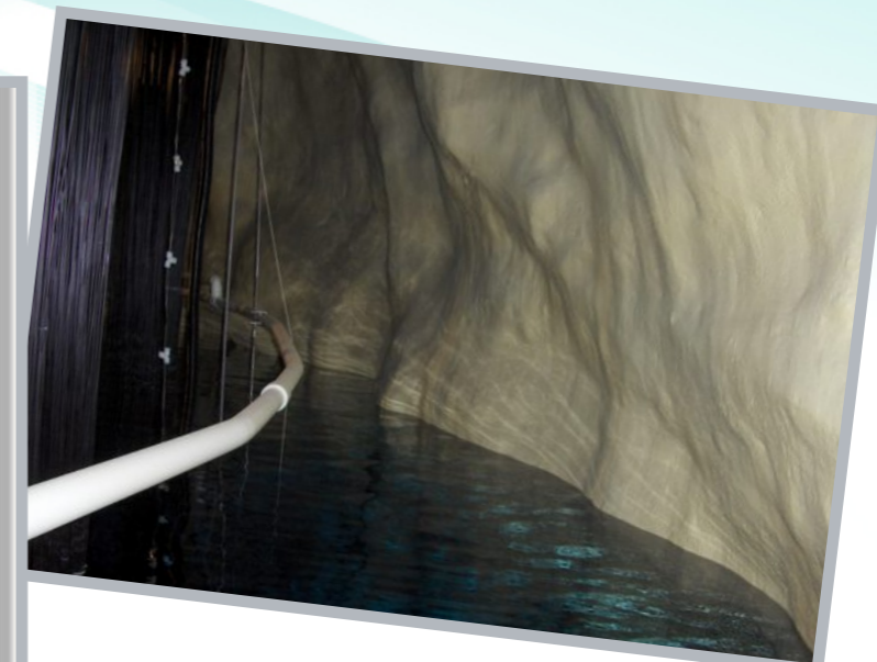
cavity wall, PMT HV cables and water
