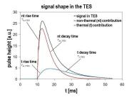
signal shape in the TES of a cryogenic detector with the TES directly deposited on the surface
