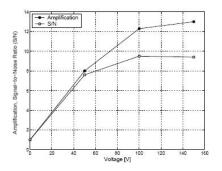
$\Rightarrow$  improvement of the signal-to-noise ratio by a factor of 10!
