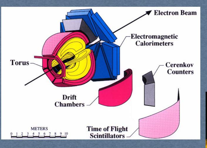
• magnetic spectrometer based on six-coil toroidal field
