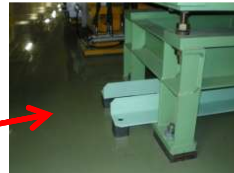
Pulling out the stage to put new longer height-adjust screws
