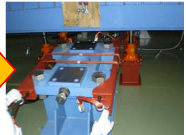
Pulling out the stage to put new longer height-adjust screws
