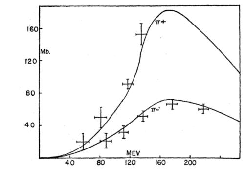
FIG. 3. Total cross sections for scattering of  $\pi^+$  and  $\pi^-$  mesons in hydrogen (including charge exchange).
