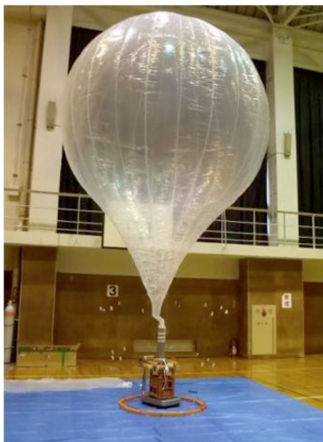
80 \mu\text{m} polyethylene test balloon
