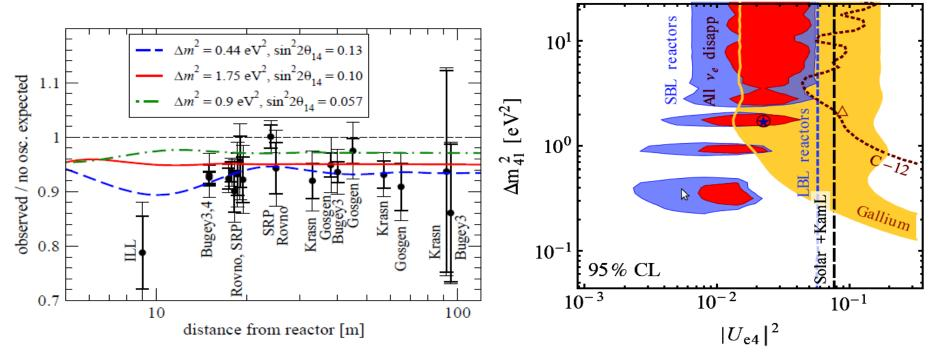
The anomaly of electron antineutrino disappearance experiments from short-baseline reactors & Gallium solar neutrino experiments may be accounted for by introducing eV scale sterile neutrinos.
