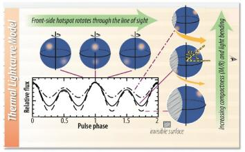
**Lightcurve modeling** constrains the compactness (M/R) and viewing geometry of a non-accreting millisecond pulsar through the depth of modulation and harmonic content of emission from rotating hot-spots, thanks to gravitational light-bending...
