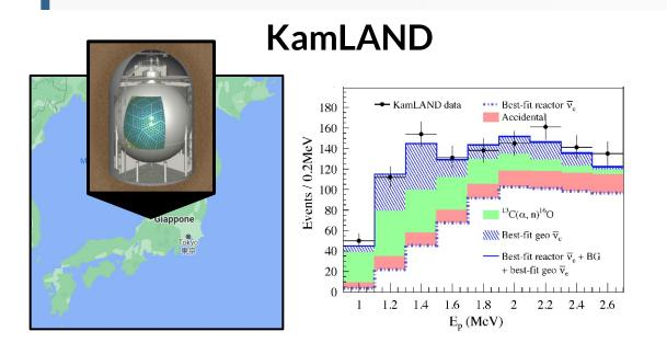
**KamLAND** is a **1 kton** liquid scintillator detector situated in **Japan**, in the Kamioka mine. It is surrounded by 1325 17" PMTs and 554 20" PMTs
