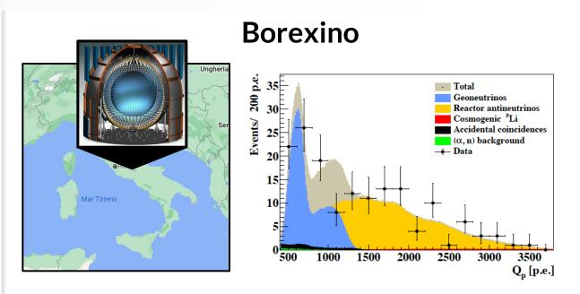
**Borexino** is **0.3 kton** liquid scintillator detector situated in **Italy**, at the Laboratori Nazionali del Gran Sasso. It is surrounded by ~2200 8" PMTs.
