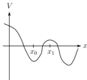
►  $\left. \frac{dV}{dx} \right|_{x=x_0} = 0, \quad \left. \frac{d^2V}{dx^2} \right|_{x=x_0} \equiv k > 0$
