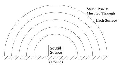
The sound power produced by the source moves outwards, and has to go through each halfsphere. Since the area of the half-spheres gets larger, the sound is being "stretched out" over a larger and larger area, and will not sound as large.
