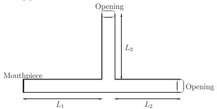
The pipes are all cylinders, 1 cm in radius, and the musician will put a clarinet mouthpiece at the closed end labeled "mouthpiece" above. I will call the three pieces of pipe the "mouthpiece pipe" (length  $L_1$ ) and the two "branch pipes" (lengths  $L_2$  and  $L_3$ ).
