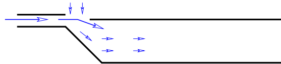
Behavior when resonance makes air flow in
