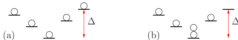
Figure 6: Schematic diagram of a single cell of the superlattice: If the superlattice amplitude \Delta is close to the interaction strength U_0 , the number states (a) and (b) have roughly the same energy. The relative height between the sites represents the different on-site energies \epsilon_i .
