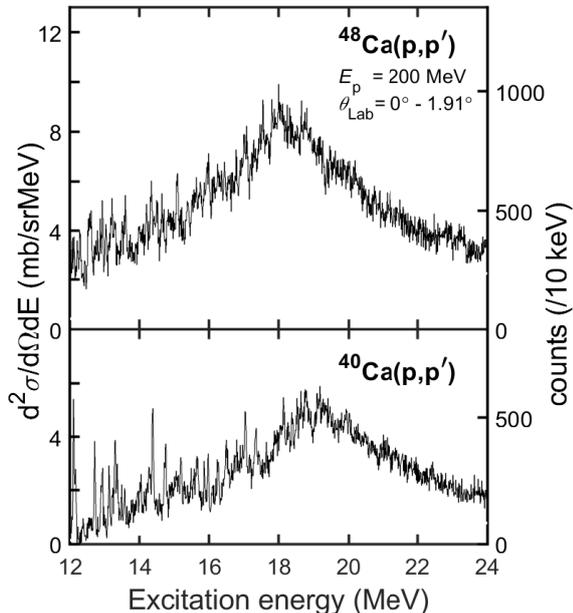
Figure 1: Spectra of  $^{40,48}\text{Ca}(p,p')$  scattering at  $E_p = 200$  MeV and scattering angles  $\theta_{\text{Lab}} = 0^\circ - 1.91^\circ$ .
